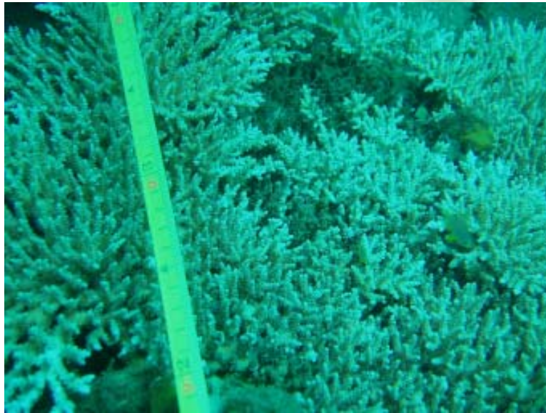
Fig. 34. The line intercept sampling method to measure disturbance-related factors, and percentage of dead and live coral cover.
